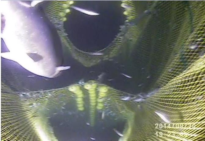
At the start of each Bering Sea EFP 15-01 test, a set of pre-test tows in mid-water (not in fish sign) were made to examine how well the shape achieved the desired parameters. Adjustments (e.g. adding floatation or leadline) were made as needed to allow the upper and lower excluder panels to come together as closely as possible at the vessel's normal towing speeds. Once the shaping was confirmed, the vessel commenced with the EFP tows.
