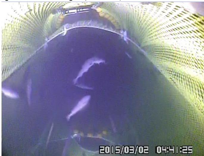
Looking at the photos, one can see the differences in size of the section in which the excluder is installed and the relative degree to which the upper and lower panels of the excluder come together. The photos also show differences in rigidity of the webbing at towing speed.
